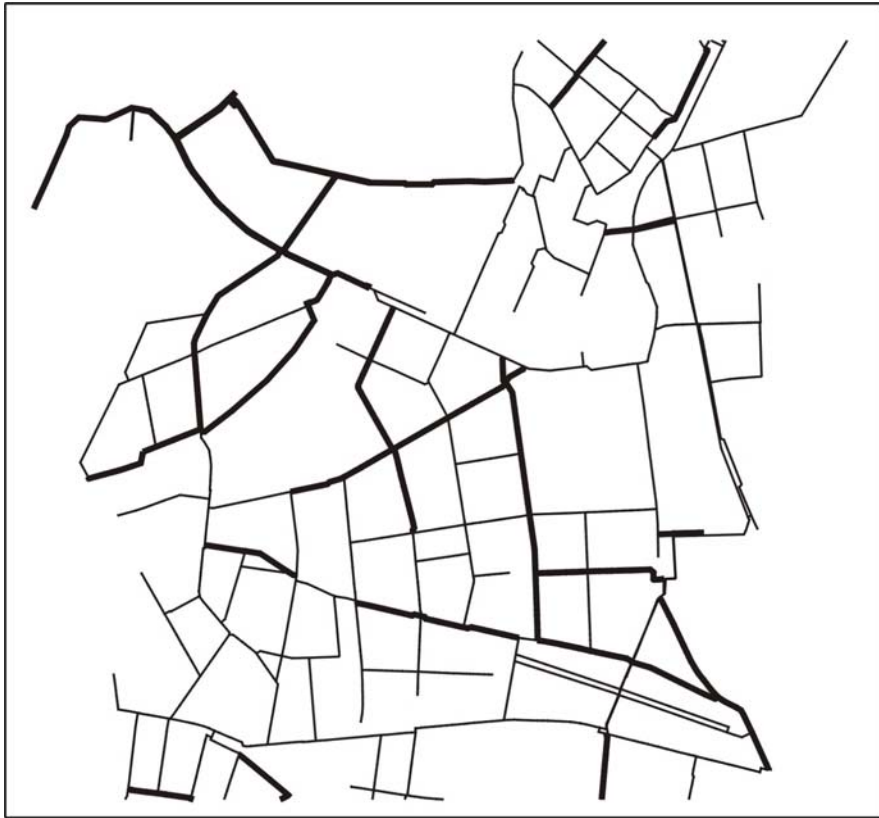
Figure 13. Detail of 1 st PZ's sub zone. The highlighted elements were classified by operators of BVK as suitable for rehabilitation (middle-term plan).
