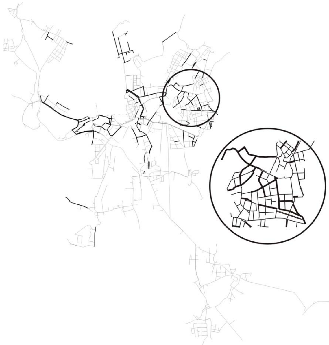
Figure 11. Water distribution network of the 1 st Brno pressure zone. Highlighted elements were classified as suitable for reconstruction during next 5 years – according to middle-term rehabilitation plan created formerly by end-user's operators. The sub zone processed by ARP module is located in the circle. Detail of the sub-zone processed by ARP.
