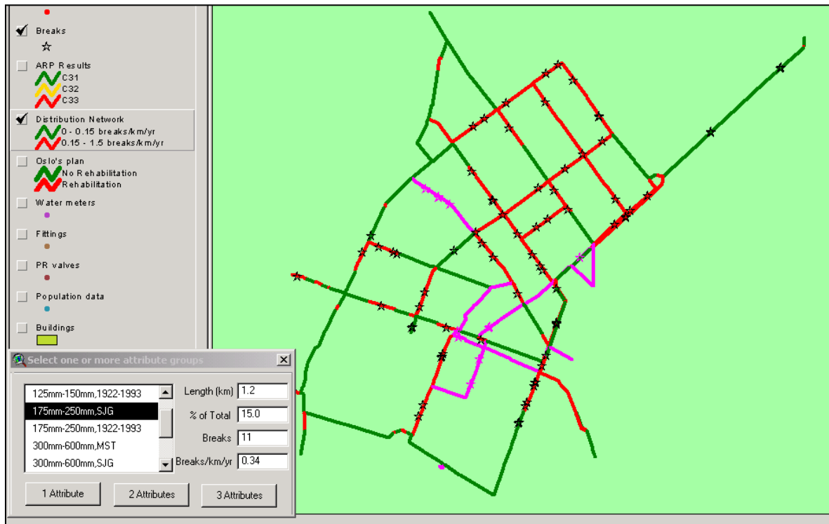
Step 4: View pipes according to their grouped attributes
