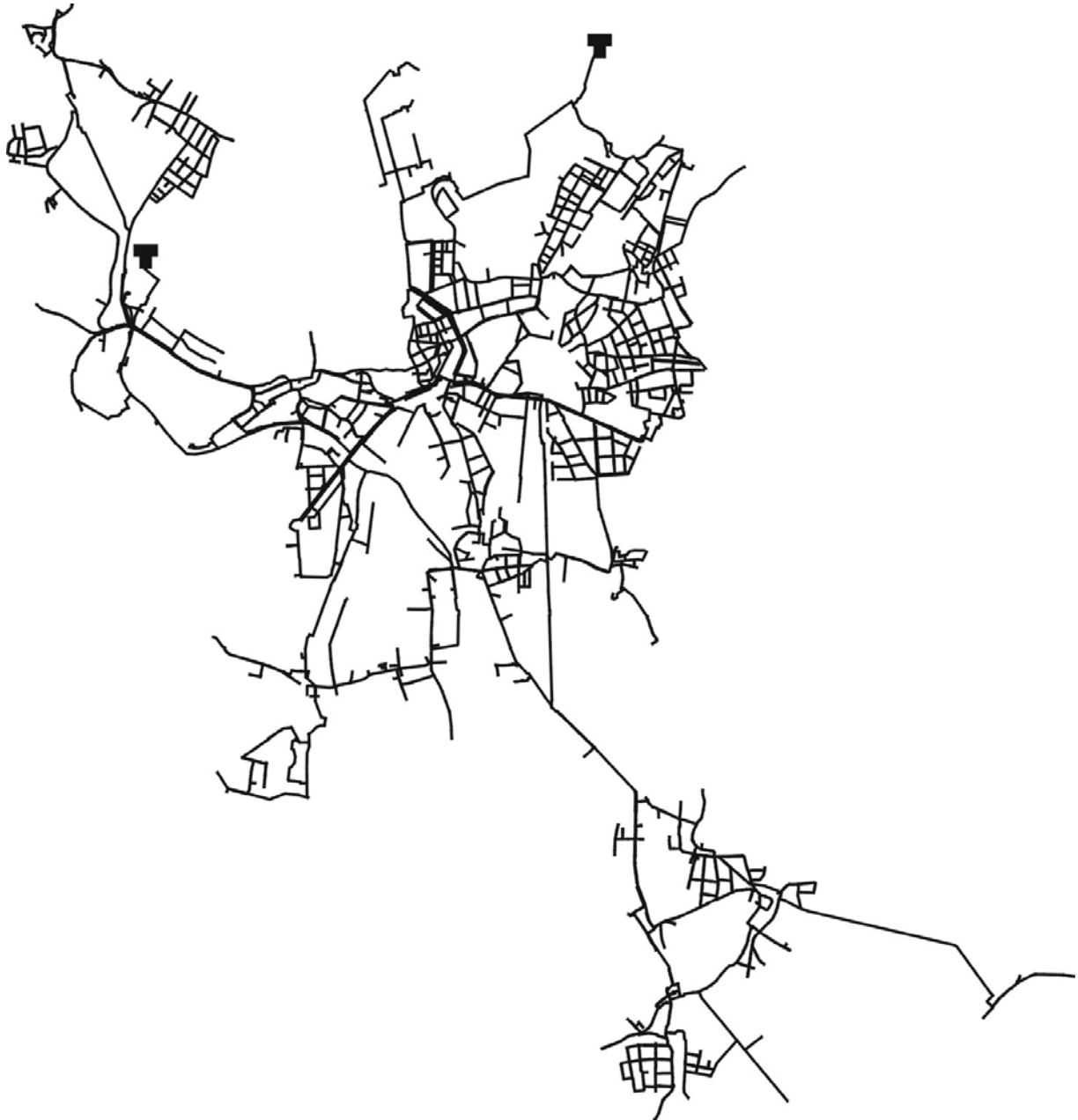
Figure 6. Hydraulic model of water distribution network of the 1 st Brno pressure zone (2,000 pipe sections, 1,631 nodes, two reservoirs – total length 267 km) used for testing RelNet.
